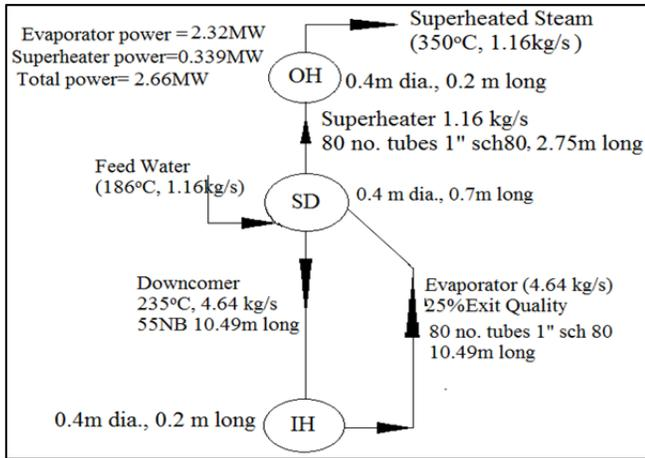
Fig. 2: Design parameters of Single SGS
