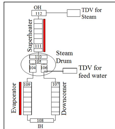
Fig. 4: Nodalization scheme used for RELAP analysis
