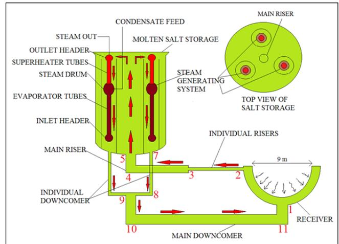
**Fig. 1: Integral Receiver System**
