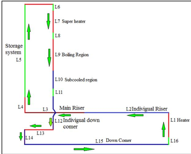
Fig. 3. The salt loop schematic used for LBENC analysis
